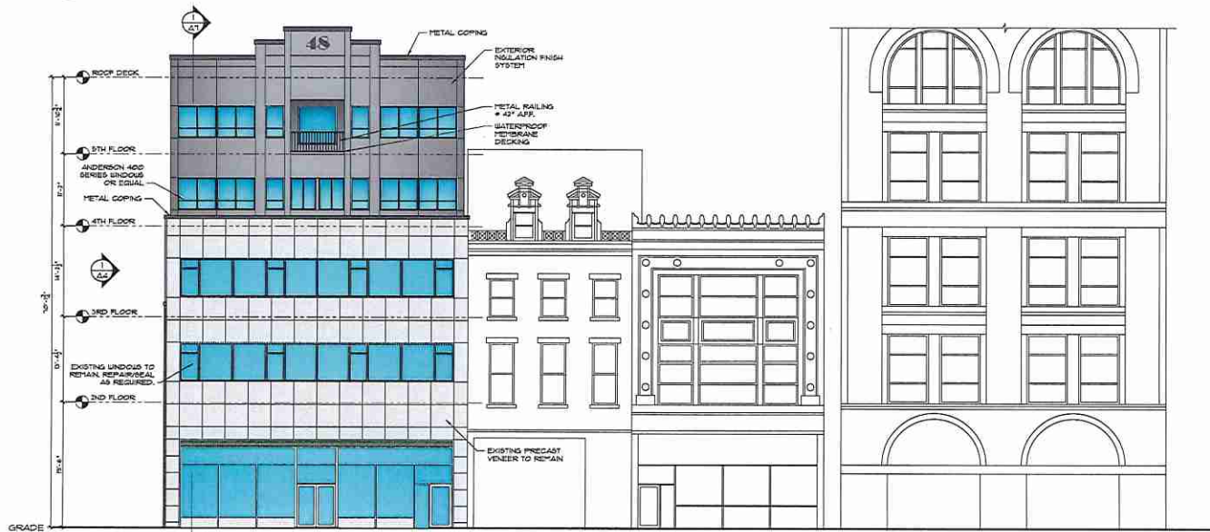
1 PROPOSED EAST ELEVATION - PEARL STREET A5 SCALE: 1/8"=1'-0"
